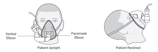
Figure 8. Connecting to a mask
