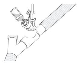
Figure 11. Filling the nebulizer with a pre-filled ampoule
