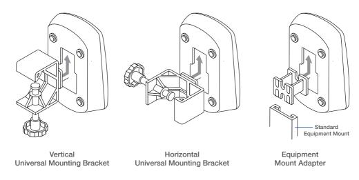
Figure 3. Aeroneb Pro-X Controller and universal mounting bracket configurations
