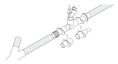
Figure 6. Connecting to a neonate breathing circuit
