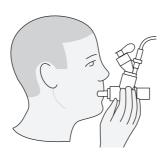
Figure 9. Connecting to a mouthpiece
