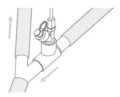
Figure 5. Connecting the Aeroneb Solo to a breathing circuit
