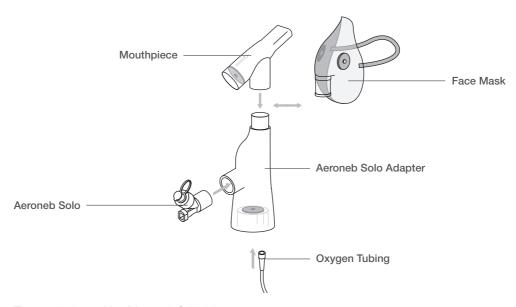
Figure 10. Assembly of Aeroneb Solo Adapter
