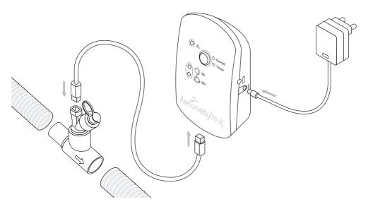
Figure 2. Assembly of Aeroneb Solo System
